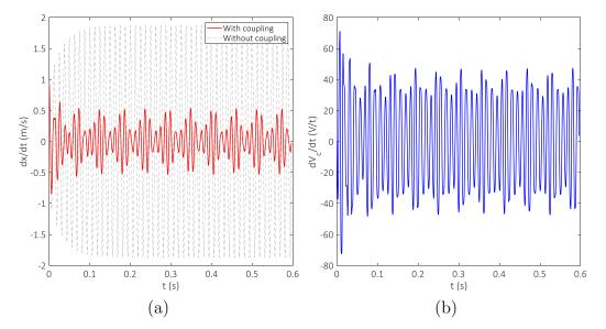
Figure 14: (a) Comparison of velocity histories as a function of time t(s) obtained by numerical integration of the system under  $L_p = 132$  dB between the master system (The loudspeaker) coupled with the NES (the shunt nonlinear circuit) represented in solid line and without NES in dotted line. (b) Histories of the voltage derivative in terms of time t(s).
