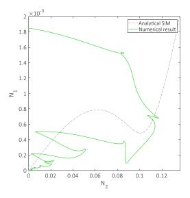
Figure 8: Invariant manifold of the system at the fast time scale  $\tau_0$  (black curve) and its corresponding numerical results (green curve) for the system under free oscillations P(t) = 0 and  $\sigma = 0$ . Numerical results correspond to the integration of System (10) versus t for  $t \in [0, 0.15]$  with the initial conditions  $x(0) = V_c = \dot{V}_c = 0$  and  $\dot{x}(0) = 1.9 \times 10^{-3}$  m s<sup>-1</sup>.
