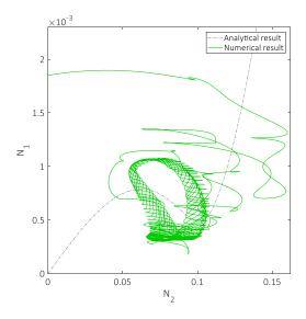
Figure 13: System invariant manifold and its corresponding numerical result for  $L_p = 132$  dB and  $\sigma = 0$ . The numerical result corresponds to the integration of System (10) with the initial conditions corresponding to  $x(0) = V_c = \dot{V}_c = 0$  and  $\dot{x}(0) = 1.9 \times 10^{-3}$  m s<sup>-1</sup>. Here, the system present a SMR illustrated in Figure 10 with two dots.
