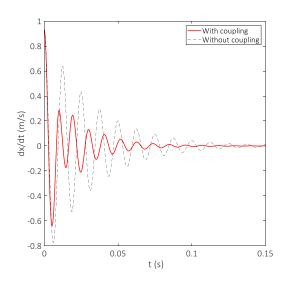
Figure 9: Histories of displacement in terms of time t(s) obtained by numerical integration of the system under free vibrations,  $\sigma = 0$  with the initial conditions corresponding to  $x(0) = V_c = \dot{V}_c = 0$  and  $\dot{x}(0) = 1.9 \times 10^{-3}$  m s<sup>-1</sup>. Dashed and full lines denote the cases of open circuit and shunt nonlinear circuit respectively.
