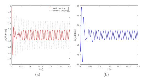
Figure 12: (a) Comparison of velocity histories as a function of time t(s) obtained by numerical integration of the system under  $L_p = 120$  dB between the master system (The loudspeaker) coupled with the NES (the shunt nonlinear circuit) represented in solid lines and without the NES in dotted line. (b) Histories of the voltage derivative in terms of time t(s).
