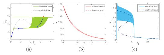
Figure 7: (a) Efficient passive TET to the NES for the case of free oscillations with initial conditions corresponding to a fixed point on the upper branch of the SIM. (b) and (c) show a comparison of energy flow between the numerical integration of the initial differential System (10) in full lines and the analytical results obtained by solving Equation (31) in dashed lines.
