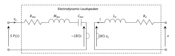
Figure 2: Circuit representation of an electrodynamic loudspeaker [8].
