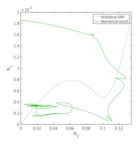
Figure 11: System invariant manifold and its corresponding numerical result for  $L_p = 120$  dB and  $\sigma = 0$ . The numerical result corresponds to the integration of System (10) with the initial conditions corresponding to  $x(0) = V_c = \dot{V}_c = 0$  and  $\dot{x}(0) = 1.9 \times 10^{-3}$  m s<sup>-1</sup>. In this case, the system is attracted by the periodic regime that corresponds to the fixed point marked with a triangle in Figure 10.
