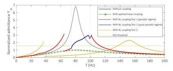
Figure 17: Comparison of the normalized admittance as function of frequency between the cases of open circuit, optimal linear resistor and the shunt nonlinear circuits. Test 1 for  $L_p = 132$  dB and Test 2 for  $L_p = 115$  dB both for k = 3468 V<sup>-2</sup>.
