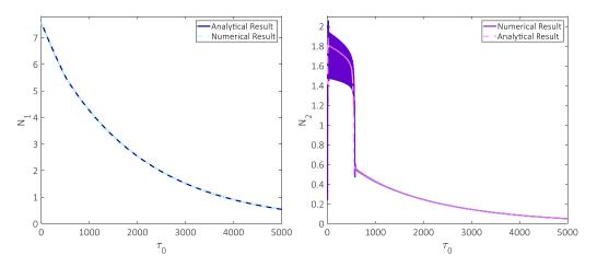
Figure 4: Numerical and analytical results for  $N_1$  and  $N_2$  during free vibrations.
