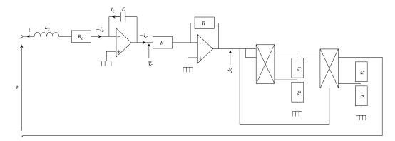
Figure 3: Nonlinear resonant circuit shunting.
