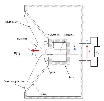
Figure 1: Shunt loudspeaker [22]
