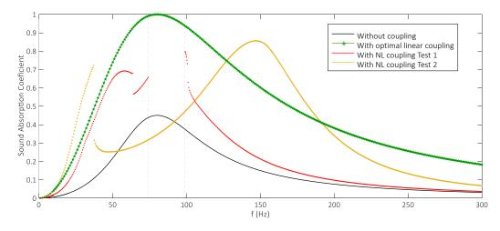
Figure 18: Comparison of the sound absorption coefficient as function of frequency between the cases of open circuit, optimal linear resistor, the shunt nonlinear circuits Test 1 for  $L_p = 132$  dB and Test 2 for  $L_p = 115$  dB both for k = 3468 V<sup>-2</sup>.
