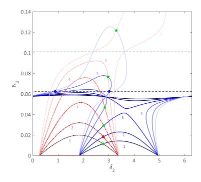
Figure 10: Positions of equilibrium points marked with stars for the system under several values of sound pressure levels  $L_p = \{116, 120, 124, 128, 132, 136\}$  (dB) for the detuning parameter  $\sigma = 0$ .  $g(N_2) = 0$  corresponds to the dotted horizontal black lines  $N_{21}$  and  $N_{22}$ .  $f_1(\delta_2, N_2) = 0$  and  $f_2(\delta_2, N_2) = 0$  are represented in dash-dotted and full line curves respectively.
