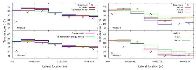
Figure 6: Separate influence of momentum and energy mixing models in Test 1.
