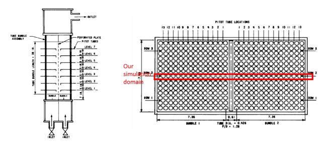
Figure 10: Test assembly and cross section of assembly (scanned from the report of Weiss [7]).
