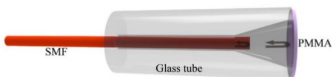
Figure 11. Schematic of FP interferometer. The FP cavity is formed by the end of fiber and PMMA film. Reprinted from [109] with permission from the Optical Society(OSA) publishing.
