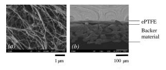
Fig. 4. Scanning Electron Microscopy analysis of the double-sided membrane. (a) Pore distribution on the Teflon side. (b) Cross-section thickness distribution with 40  $\mu$ m Teflon and 150  $\mu$ m backer material (polypropylene for Aspire QP955 and polyester for Aspire QL217).
