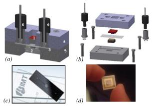
Fig. 7. (a) Longitudinal cross-section: (1) – laser diode, (2) – CMOS sensor,
