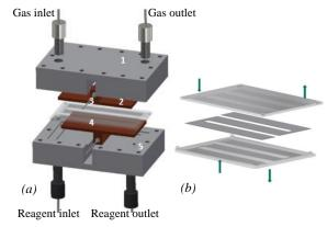
Fig. 3. (a) (1) – Holder. (2) – Copper layer. (3) – Cartridge heater. (4) – Gas-liquid contacting chip. (5) – O-ring. (b) Gas-liquid polymer contactor: exploded view.
