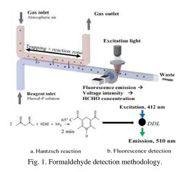
The Hantzsch reaction is a derivatization process of the formaldehyde molecules into 3,5–diacetyl-1,4dihydrolutidine (DDL), a fluorescent chemical compound. The fluoral-P or acetylacetone based solutions are used as reagents for the derivatization process, once the formaldehyde molecules are trapped into the solution. This technique is a very sensitive and a relatively simple tool to detect formaldehyde.
