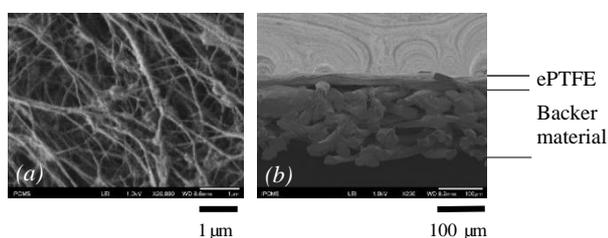
Fig. 4. Scanning Electron Microscopy analysis of the double-sided membrane. (a) Pore distribution on the Teflon side. (b) Cross-section thickness distribution with 40  $\mu\text{m}$  Teflon and 150  $\mu\text{m}$  backer material (polypropylene for Aspire QP955 and polyester for Aspire QL217).
