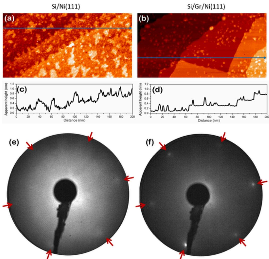
Fig. 6. STM images of 1 ML Si deposition at RT on (a) Ni(111) ( $200 \times 100$  nm, 0.1 V, 5 nA) and (b) Gr/Ni(111) ( $200 \times 100$  nm, 0.02 V, 100 nA). Panels (c) and (d): Line profiles taken along the blue lines in (a) and (b), respectively. Panels (e) and (f): Corresponding LEED patterns. Red arrows indicate the position of the faint substrate bulk spots. (A colour version of this figure can be viewed online.)
