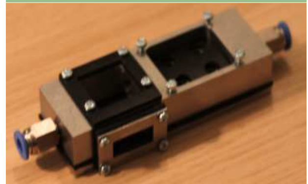
Fig. 3. Top: functional sketch of the full sensor cell bottom. The mylar membrane is in the bottom left part while, in the upper right part, four commercial sensors are installed. Bottom: corresponding realized cell
