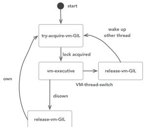
**Figure 2. Illustrated life-cycle of a VM thread in the presence of VM thread-switch.** When a green thread affined to a VM thread different than the current one is scheduled to run, the current VM thread releases the GIL and the affined VM thread is awoken.
