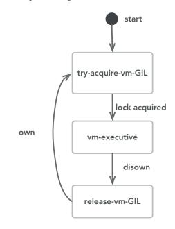
**Figure 1. Illustrated life-cycle of a VM thread in the presence of I/O.** The GIL is acquired before entering the vm-executive, and released on I/O operations. When the I/O operation finishes the VM thread attempts to re-acquire the GIL.
