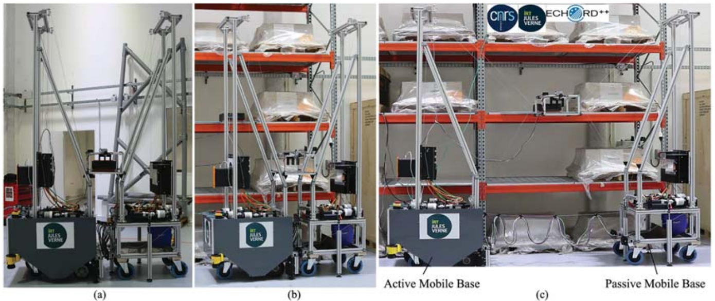
Fig. 1. FASTKIT prototype (a) Navigation mode (b) Undeployed configuration (c) Deployed configuration at the task location
