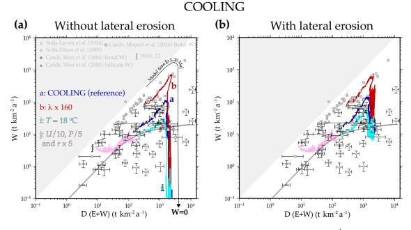
**Figure 7.** Different experiments with cooling climate. The temperature decreases with elevation  $(-6 \,^{\circ}\text{C km}^{-1})$ , the sea level temperature *T* decreases by 8  $^{\circ}\text{C}$  in four steps, and the rainfall decreases -5% per degree of cooling. Experiments a (COOLING), b, i, and j use the same parameters as in Fig. 4 but with a cooling climate. Without (a) and with ( $\alpha = 0.001$ ) (b) lateral erosion.
