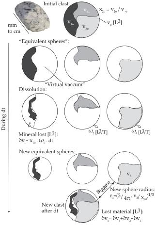
**Figure 1.** The dissolution model for a clast made up of three different mineral types. The sequence from top to bottom illustrates the mineral dissolution and the resulting clast size decrease during a time step.
