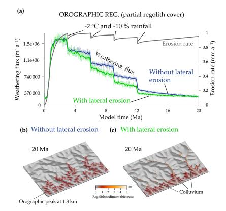
**Figure 10.** Same as Fig. 9 (cooling ending with a regolith at elevations < 1500 m), but the precipitations vary with elevation according to a Gaussian curve with an elevation peak at 1300 m (orographic model 1 illustrated in Fig. 8). The erodibility parameters (Eq. 2) are also doubled to compensate for the smaller precipitation rate at high elevations and thus to obtain comparable maximum elevations.
