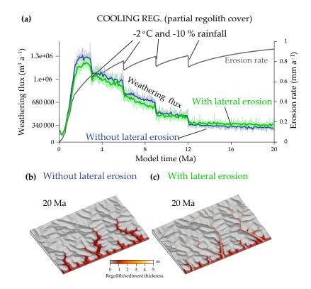
**Figure 9.** Experiments ending with a regolith covering the low elevations (< 1500 m) and corresponding to a cooling climate. (a) Erosion and weathering flux through time for the models without and with lateral erosion. Panels (b) and (c) show corresponding topography and regolith or sediment thickness at 20 Ma for the model with and without lateral erosion.
