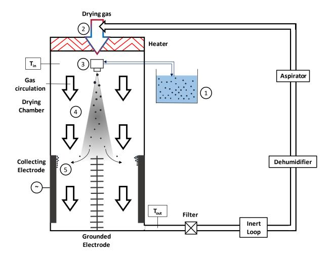
Figure 1: Flowsheet of the nano spray-drying process (adapted from <sup>31</sup>).
