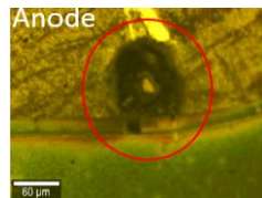
Fig. 7: Optical microscopy after high voltage failure on the corner of the device
