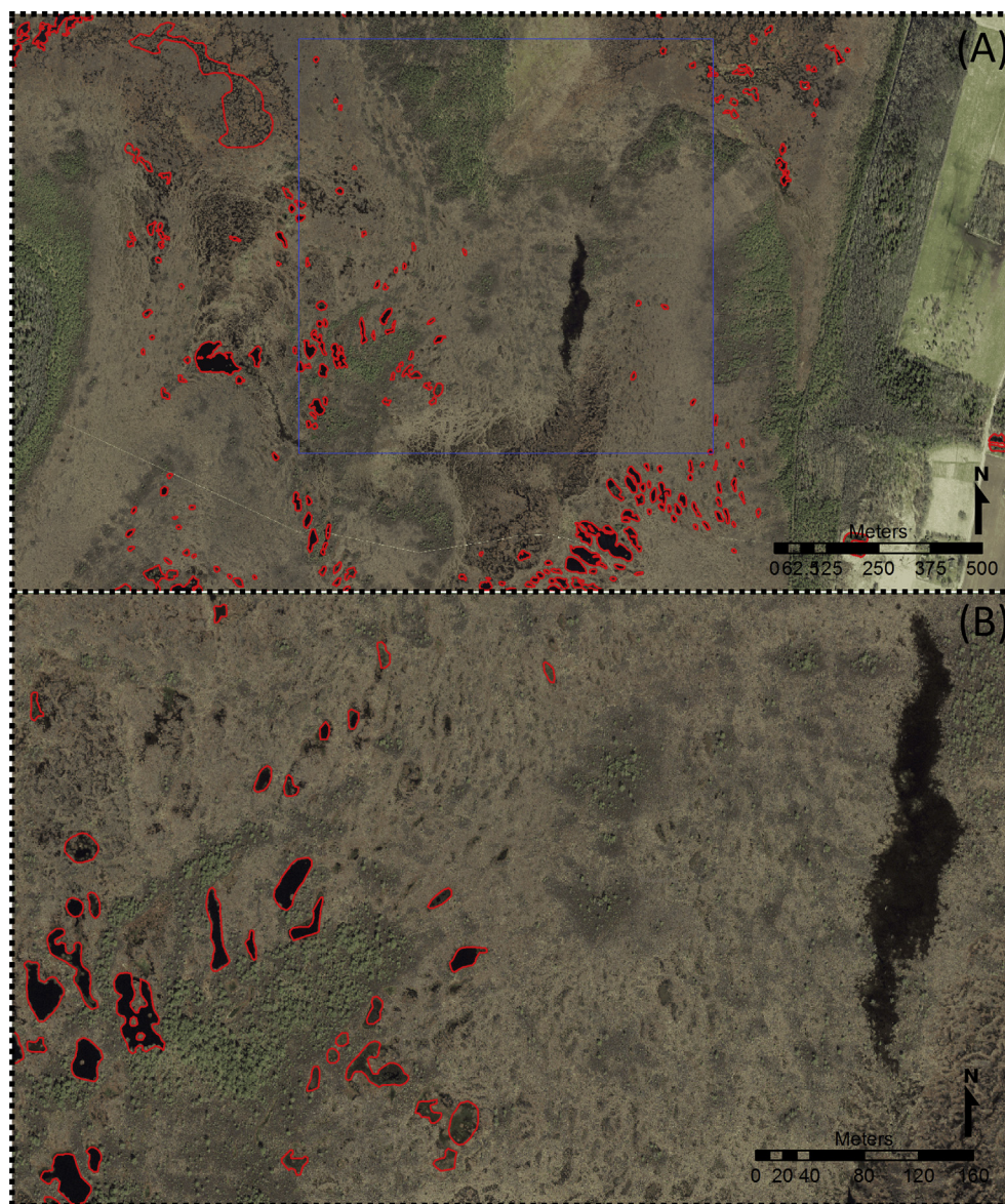
Fig. 2. Discrepancies in bog pool data in the Nigula Bog (Estonia). (A) The blue square is one of the randomly selected 1 × 1 km plots. Red contours are SWBs from Estonian Topographic Database (ETD). (B) Several bog pools visible in the Estonian Land Board orthophoto are missing from the database, whereas some bog pools marked in ETD have almost disappeared.
