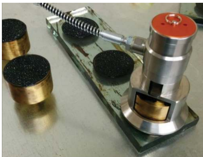
Fig. 2. Brass pull-stub (50 mm diameter) with 4 cuts (13 mm) along the perimeter edge and 0.3 mm edge.
