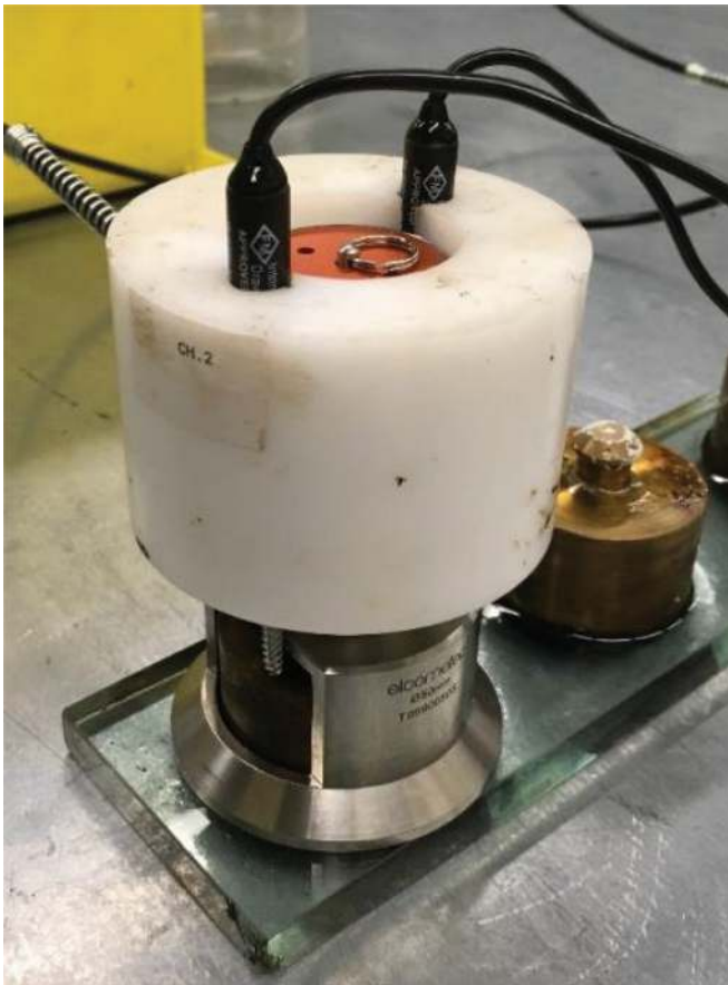
Fig. 5. Modification of the pull-off test device to include two LVDTs for displacement measurements. [Colour online.]
