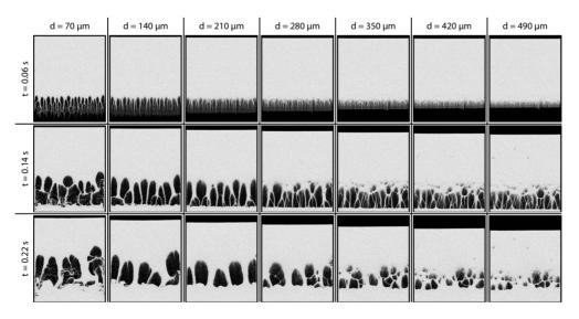
FIG. 2. Numerical snapshots. Each column represents different simulations using grains of diameter d, and each row represents snapshots at different times t.
