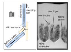
FIG. 1. (Color online) (left) Side view of the experimental setup with the initial and final cell positions superimposed. (right) Typical snapshot from an experiment using grains of 230  $\mu$ m in diameter in a cell that is 91×141×2.3 mm.
