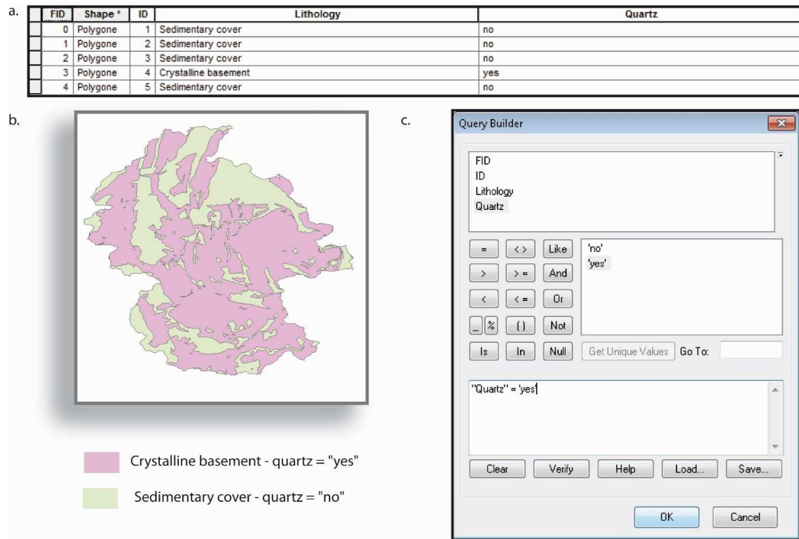
Fig. D: a. Example of an attribute table providing lithological information and specifying the presence or absence of quartz in an independent field (e.g. the field named 'Quartz'); b. Example of a shape file showing the polygons associated with the attribute table where the lithological information is given (after Delunel et al. (2010)); c. SQL interface open once the correction for lithology is selected. To compute the production rate in the region with quartz only (e.g. 'Crystalline basement') the user must specified a SQL expression (e.g. 'Quartz' = 'yes') which selects the correct polygons from the shape file accordingly.
