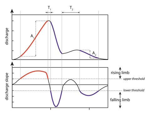
**Figure 1.** Conceptual view of the algorithm developed to identify a storm event in discharge time series. A<sub>i</sub>: storm event amplitudes, T<sub>i</sub>: time between two identified stages.
