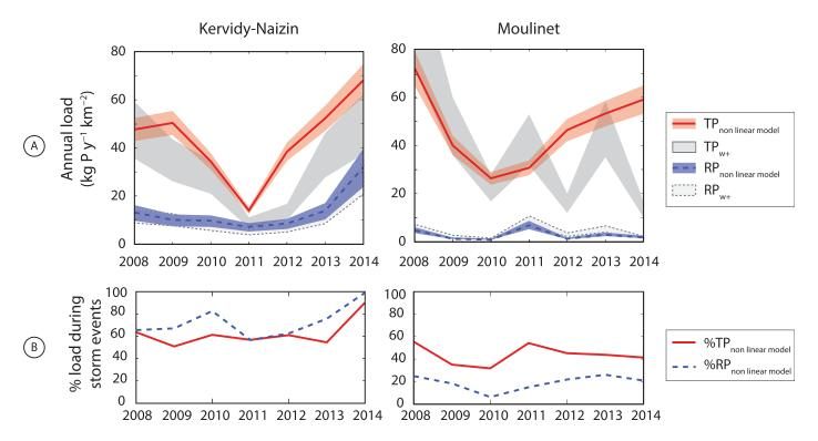
Figure 8. (a) Application of the nonlinear empirical method M3 to estimate annual TP and RP loads and compared to estimations based on a weekly+ survey without storm event reconstruction in Kervidy-Naizin and Moulinet catchments. Uncertainty ranges are based on results from Irish data sets. (b) Proportion of load occurring during storm events only.
