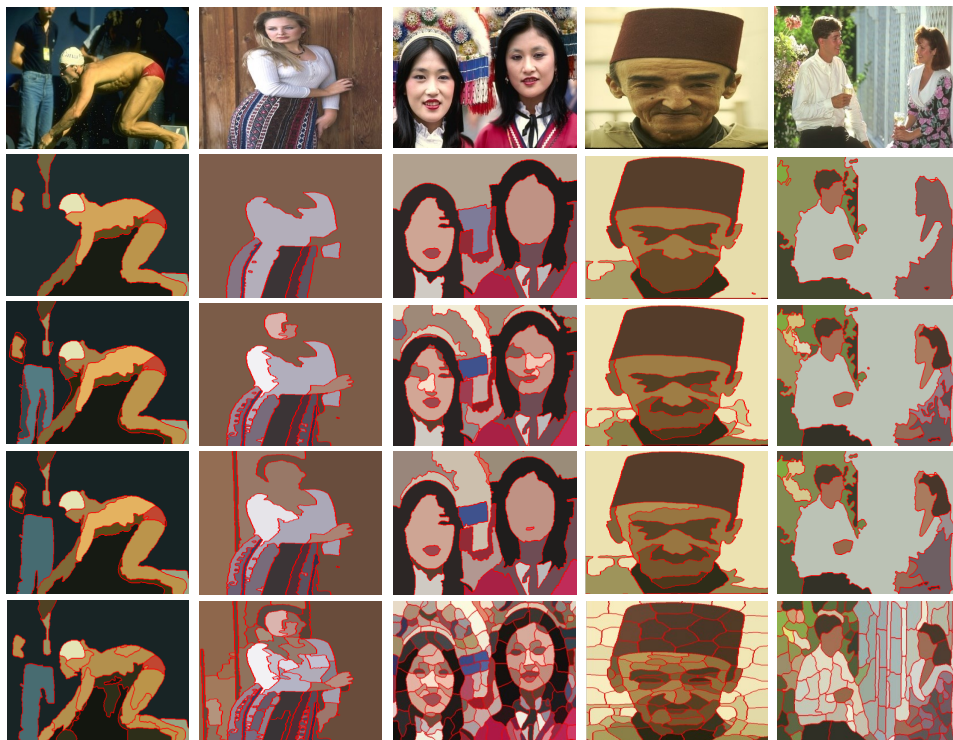
Fig. 8: Segmentation results for images from people category, Line 1:Original image; Line 2: Fast multi-scale community detection algorithm; Line 3: Fast greedy modularity optimization algorithm; Line 4: Louvain; Line 5: Infomap.
