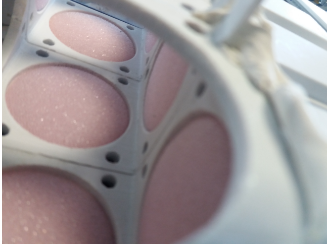
FIG. 10. View of the waveguide interior. The layers of foam, in pink color applied in front of the loudspeakers, do not interfere with the diaphragms mechanical vibration. The "flush" condition of the liner is maintained.
