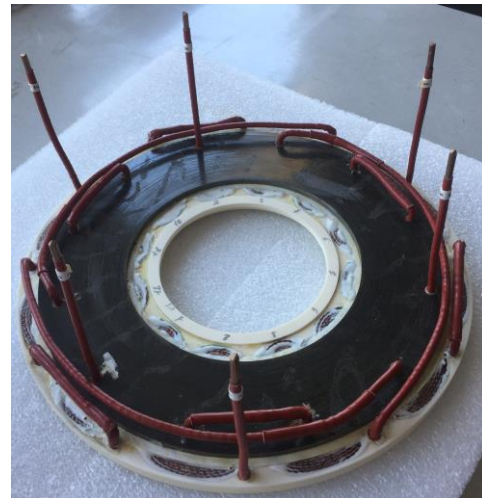
Fig. 10. Static cryostat with the armature winding
