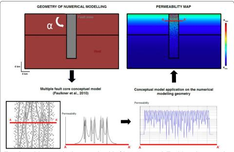
**Fig. 5** Permeability imposed in the numerical models of the parametric study. The alpha angle corresponds to the dip of the fault zone (here  $\alpha = 90^{\circ}$ ). The permeability of the basement and fault will decrease with depth according to Eq. 6 (Garibaldi et al. 2010). Within the fault zone, permeability will also vary laterally (Eq. 7) to match field observations
