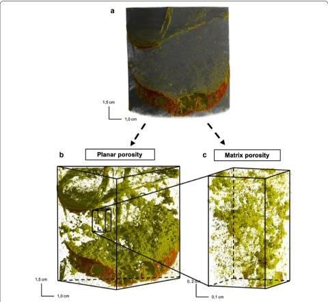
**Fig. 9** Three-dimensional observations of the planar and matrix porosity of one sample taken from the Pontgibaud fault zone. The red color of figures **a**, **b** corresponds to mineralization (lead sulphides). The yellow color of figures **a**, **b** corresponds to the planar porosity located on the fracture walls. The yellow color of figure **c** could correspond to the matrix porosity. The resolution of figures **a**–**c** is, respectively, 25, 25 and 4 μm
