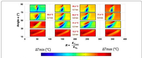
**Fig. 11** Graphical representation of all numerical models of temperature anomalies on the theoretical fault zone performed (n = 216). The values of positive thermal anomalies are shown in red. Their depths are represented in brown
