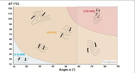
**Fig. 12** Diagram of convective regimes. Grey lines represent isotherm morphology. The dashed black line separate three area. In blue, the area of unicellular weak type convection zone. In orange, the area of unicellular medium-type convection zone. In red, the area of bicellular strong-type convection zone. The dashed grey contour on the right of the diagram illustrates the possible range for the Pontgibaud fault zone
