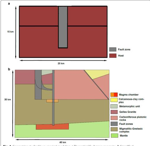
**Fig. 4** Geometries studied by numerical modeling. **a** Theoretical fault zone geometry. **b** Simplified crustal-scale geometry containing essential structural elements derived from field and geophysical data, and MT interpretation
