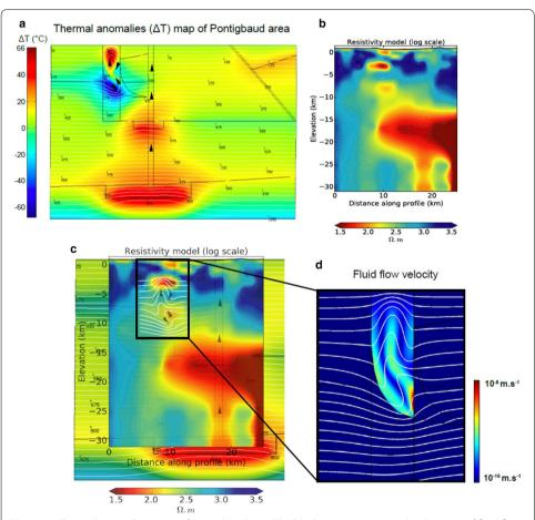
**Fig. 14** a Thermal anomalies maps of Pontgibaud area. The black arrows represent the direction of fluid flow. **b** Resistivity model previously described (Fig. 3). **c** Comparison of the numerical simulation result affecting a  $K_{\rm fmax}$  permeability of  $1.6 \times 10^{-14}$  m<sup>-2</sup> at the Pontgibaud fault zone, with the resistivity profile. **d** Fluid flow velocity within the Pontgibaud fault zone
