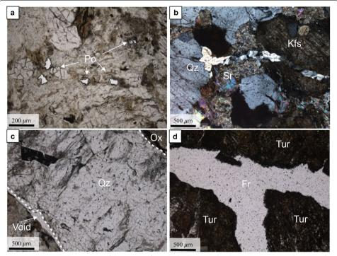
**Fig. 8** Microscopic observations of thin-section from the hydrothermalized zone. **a** Anatexite rich in veins. **b** Fractured anatexite. **c** Mineralized breach. **d** Porous breach. (Po) Porosity. (Qz) Quartz. (Void) Void. (Fr) Fracture. (Tur) Turmaline. (Ox) Oxide. (Sr) Sericites. (Kfs) Potassic feldspar
