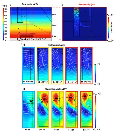
**Fig. 13** Maps of temperatures (**a**), permeabilities (**b**), isotherms (**c**), and thermal anomalies (**d**) of the Pontgibaud region (at time  $t_0+15,000$  years). In accordance with Fig. 11, color of boxes contours correspond to one convective regime: blues boxes correspond to areas of unicellular weak-type convection zone, oranges boxes correspond to unicellular medium-type convection zone, and reds boxes correspond to bicellular strong-type convection zone
