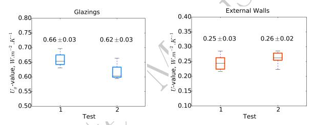
**Figure 2.** Local U-values. Each boxplot corresponds to the U-values estimated for each QUB/e test for the glazings (left) and the external walls (right).
