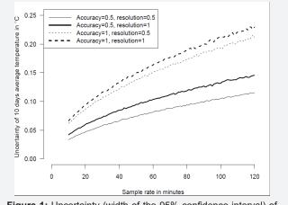
**Figure 1:** Uncertainty (width of the 95% confidence interval) of the average temperature for 10 days dependent on the accuracy and resolution of the data logger for one measure and the sample rate in minutes.
