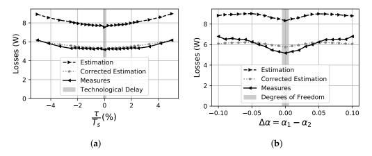
**Figure 14.** Estimated, Estimated after correction and Measured Losses under (**a**) delay and (**b**) duty-cycle difference.
