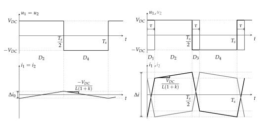
**Figure 5.** Voltage and Current Evolution under (**a**) synchronised control signals, (**b**) a delay between control signals.
