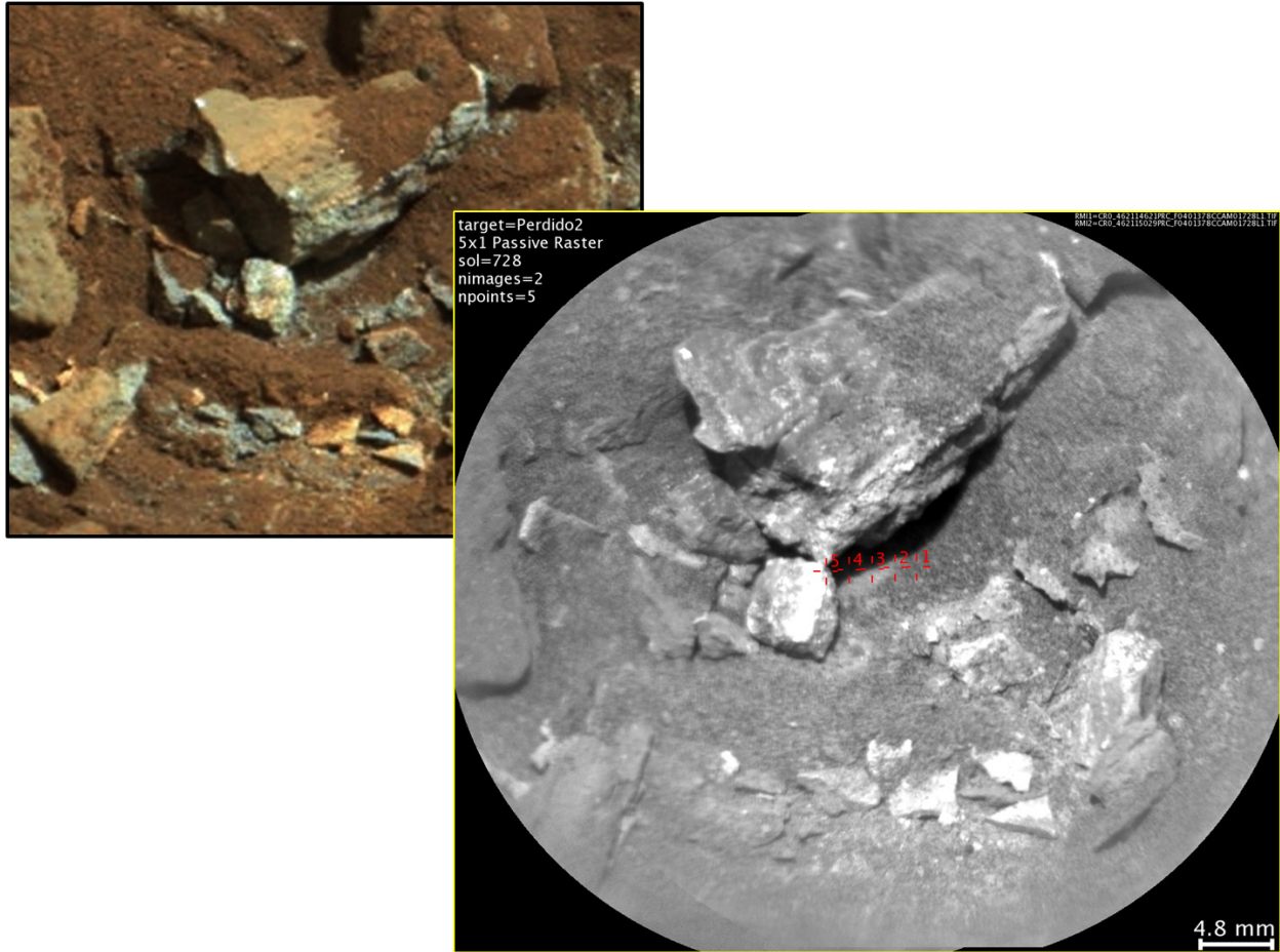
824 Figure 4. Portion of Sol 725 Mastcam M-100 image (0725MR0030940000402844E01) showing 825 Perdido2 target, along with Sol 728 RMI mosaic (ccam01728; CR0_462114621, 826 CR0_462115029) showing 5x1 ChemCam passive raster locations. This was acquired after a 827 ChemCam LIBS observation on Sol 725 (sequence 3725) on the broken rock Perdido (directly 828 above this raster) exhibited passive spectra (3 msec “dark” exposures) with a potential 433 nm 829 absorption band.
