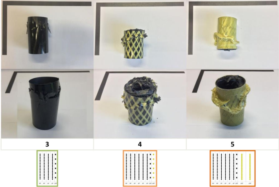
Figure 26: Pictures of CFRP tubes specimen 3, 4 and 5 which underwent catastrophic failure for inner-crushing configuration (b).
