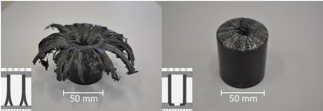
Figure 17: Crushed CFRP tubes (1) showing outer spreading (left) and inner folding (right) based on boundary condition (a) free crushing and (b) Inner crushing, respectively.
