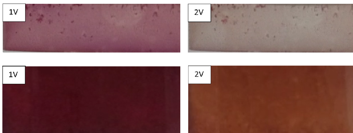
Fig. 6. Pictures of FTO substrates modified with poly-2 grown in (top) 1 mM and (bottom) 3 mM solution in (left) reduced form at 1 V vs Ag/AgCl and (right) oxidized form at 2 V vs Ag/AgCl. Potential variation was made in 0.5 M tetraethylammonium tetrafluoroborate (TEABF 4 ) acetonitrile solution.
