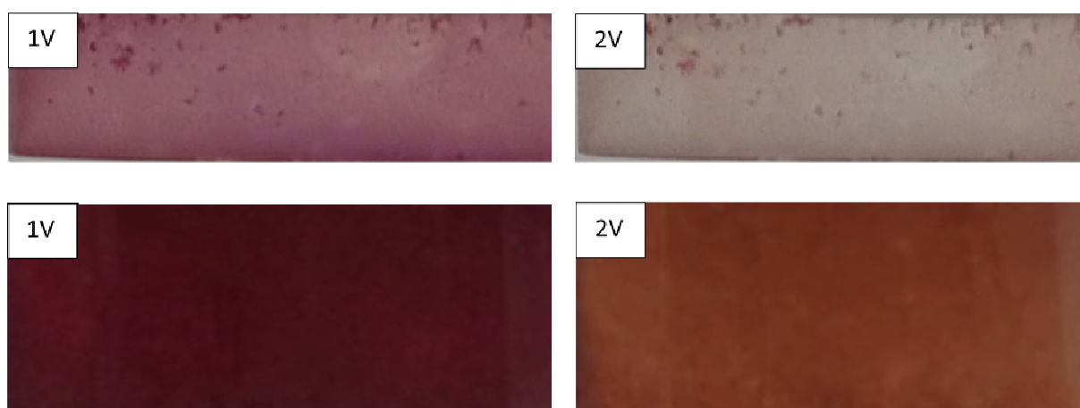
Fig. 6. Pictures of FTO substrates modified with poly-2 grown in (top) 1 mM and (bottom) 3 mM solution in (left) reduced form at 1 V vs Ag/AgCl and (right) oxidized form at 2 V vs Ag/AgCl. Potential variation was made in 0.5 M tetraethylammonium tetrafluoroborate (TEABF 4 ) acetonitrile solution.
