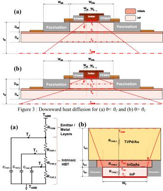
Figure 4: (a) Equivalent electro-thermal network for the vertical InP HBT architecture implemented in HiCuM compact model; (b) Thermal resistance contribution of the emitter and metal layers (upward heat-flow).
