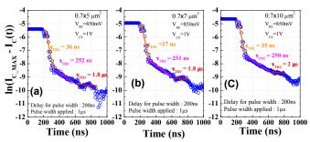
Figure 12: Extraction of thermal time constant,  $\tau_{TH}$ , from pulse measurements for the geometries with  $W_{E0}$ =0.7 $\mu$ m and  $L_{E0}$  (a) 5, (b) 7 and (c) 10  $\mu$ m.
