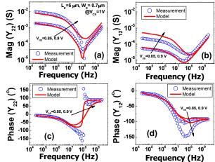
Figure 8 : Comparison between measurements (symbols) and simulation (solid lines) for (a) Y<sub>12</sub> magnitude, (b) Y<sub>22</sub> magnitude, (c) Y<sub>12</sub> phase and (d)  $Y_{22}$  phase for the geometry  $0.7 \times 5 \mu m^2$  as a function of different  $V_{BE}$  at  $V_{CE}=1V.$
