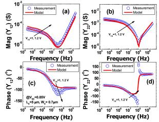
Figure 7 : Comparison between measurements (symbols) and simulation (solid lines) for magnitudes of (a) Y12, (b) Y22, and phases of (c) Y12 and (d)  $Y_{22}$  for the geometry  $0.7 \times 5 \mu m^2$  as a function of different V<sub>CE</sub> at V<sub>BE</sub>=0.85V
