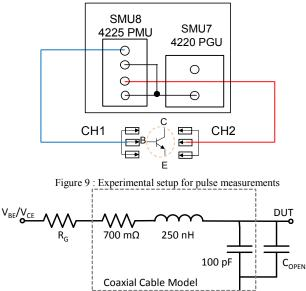
Figure 10 : Equivalent circuit model of the coaxial cables consisting of passive elements, the generator resistance  $R_G$  and device open capacitance  $C_{OPEN}$ .
