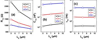
Figure 13: Extracted values of the (a)  $R_{TH}$ , (b)  $C_{TH}$  and (c)  $\tau_{TH}$  of the three regions for three geometries with  $L_{E0}$ =5,7 and 10  $\mu$ m and  $W_{E0}$ =0.7  $\mu$ m.
