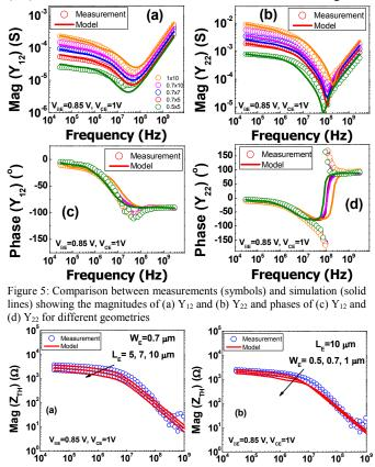
Frequency (Hz) Frequency (Hz) Figure 6 : Comparison between measurements (symbols) and simulation (solid lines) showing the magnitudes of Z<sub>TH</sub> for different (a) L<sub>E0</sub> and (b) W<sub>E0</sub>.
