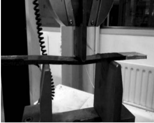
Figure 4. Static 3-point bending test on Instron 5566A bench.
