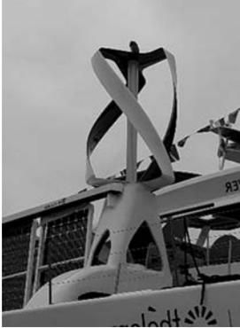
Figure 2. Energy observer wind turbine.
