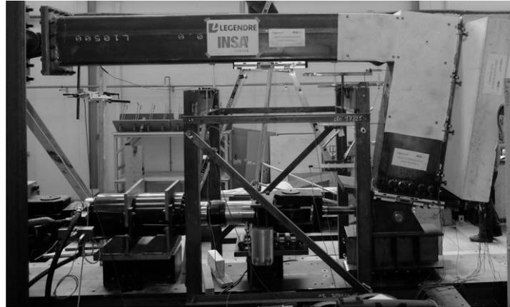
Fig. 27. Beam-column joint after collapse
