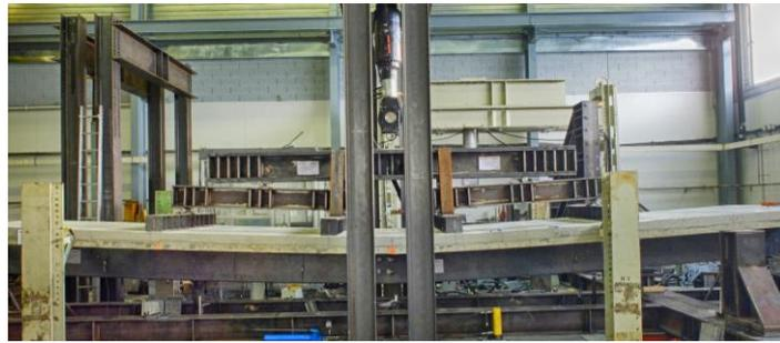
Fig. 21. Deflection of the beam after test
