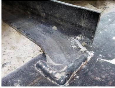
Fig. 12. Angle deformations after testing
