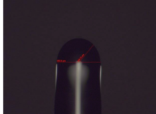
FIGURE 4. (a) Step refractive indexes of a TEQS TM coated multimode fiber. (b) Spheroid tip of 200 \mu\text{m} TEQS TM coated multimode fiber
