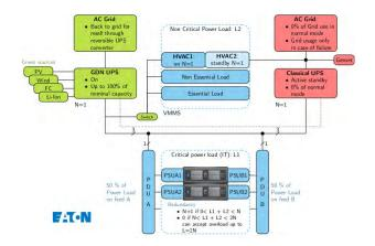
**FIGURE 1.** Classical datacenter architecture with N + 1 redundancy (Green + Grid).
