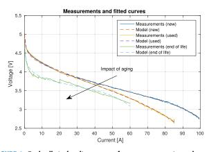
FIGURE 4. Fuel cell stack voltage curves from measurements run by FEMTO-ST/FCLAB and resulting model output for different aging levels (new, used and end of life).
