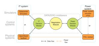
FIGURE 14. System overview, including simulators (datacenter simulator and power system simulator) and physical parts (IT OpenStack and PHIL).
