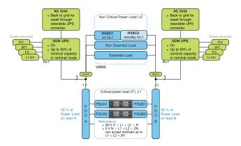
FIGURE 2. Breakthrough architecture with 2N redundancy (Green + Green).
