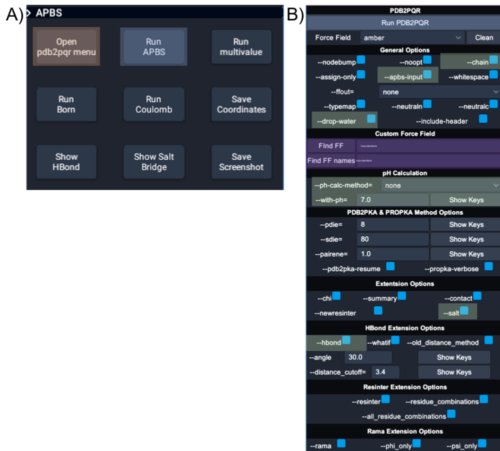
Figure 1. UnityMol-APBS user interface for PDB2PQR and APBS. (A) The main UnityMol-APBS menu; orange box highlights the two buttons used to open the APBS and PDB2PQR tools. (B) The main menu for interactions with APBS and PDB2PQR. Blue boxes show the buttons to launch PDB2PQR and APBS executables, green boxes show the location of the options used for producing the images in Figures 2 and 3, and the purple boxes highlight the two input fields required to use custom force fields and custom residue names.
