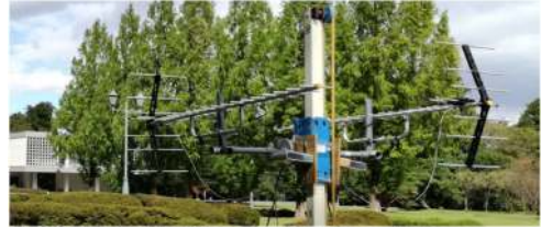
Fig. 21. Reference and surveillance antennas are both mounted on the rail.
