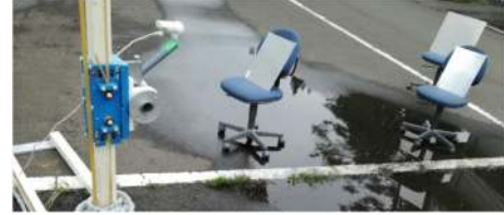
Fig. 16. Detection of three metallic plates with the surveillance antenna sledged on the positioner with a 5 mm step.
