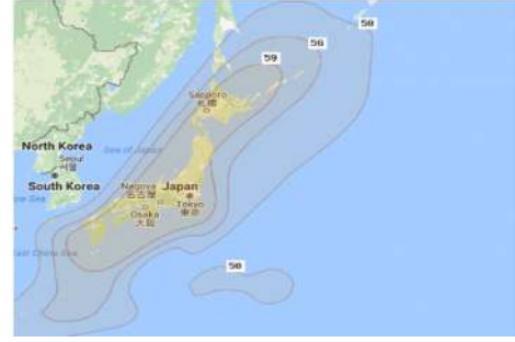
Fig. 4. Covered area of CS satellite with different Equivalent Isotropically Radiated Powers (EIRPs), provided by LyngSat website.
