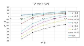
Fig. 11 Most negative Poisson's ratio values for the hexaround lattice with respect to a and  $\rho^{\star}$
