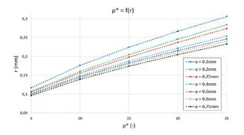
Fig. 12 Effect of the strut radius on the relative density for the inverse hexaround cell
