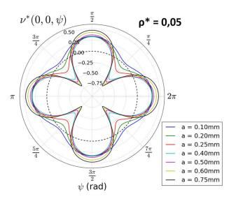
Fig. 10 Hexaround Poisson's ratio within the (100) plane, for various a and  $\rho^{\star}$  = 0.05
