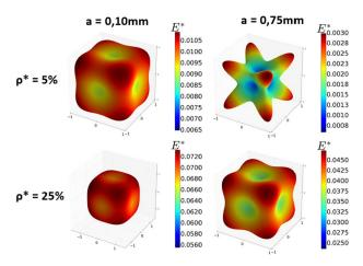
Fig. 13 3D maps of normalized Young's modulus for various relative density  $\rho^*$  and pre-buckling amplitude a for the inverse hexaround cell
