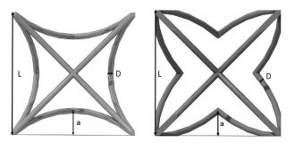
Fig. 2 Hexaround (left) and inverse hexaround (right) geometric descriptions
