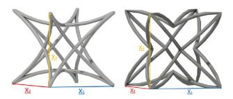
Fig. 1 Hexaround (left) and inverse hexaround (right) unit cells, with their periodicity vectors  $\underline{\mathbf{X}}_i$
