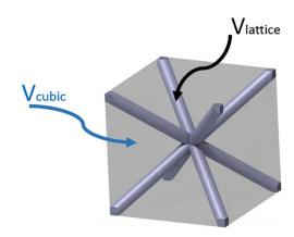
Fig. 6 Definition of  $V_{\text{lattice}}$  and  $V_{\text{cubic}}$
