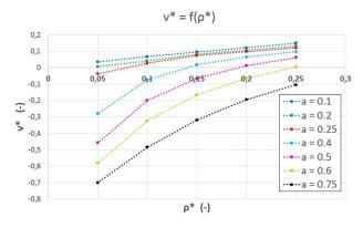
Fig. 16 Most negative Poisson's ratio values for the inverse hexaround lattice with respect to a and  $\rho^*$
