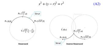
Fig. 19 Geometries used to define the struts of hexaround cell (left) and inverse hexaround cell (right)
