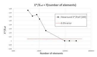
Fig. 20 Mesh sensitivity study for an hexaround cell with  $a=0.75~\mathrm{mm}$  and  $\rho^{\star}=0.10$ .  $E_{\mathrm{ref}}$  is the converged normalized Young's modulus for a high mesh density (271k elements).
