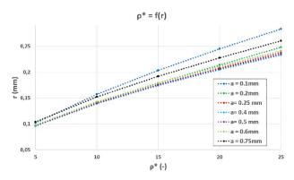
Fig. 7 Effect of the strut radius on the relative density for the
