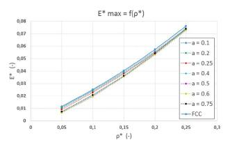
Fig. 9 Hexaround maximal effective Young's modulus with respect to relative density  $\rho^*$  and pre-buckling amplitude a
