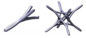
Fig. 3 1/8 of cell with intersection (left) and resulting cell (right)
