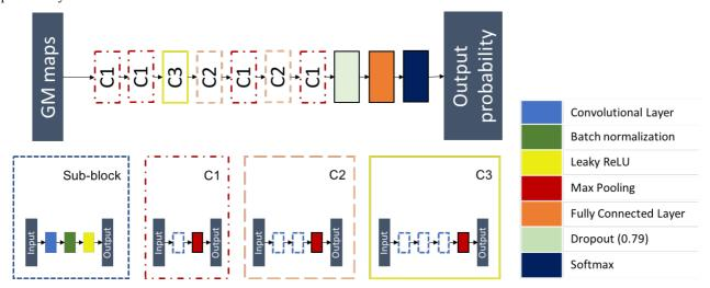
Figure 1: Architecture of the CNN classifier determined following to a random search procedure.
