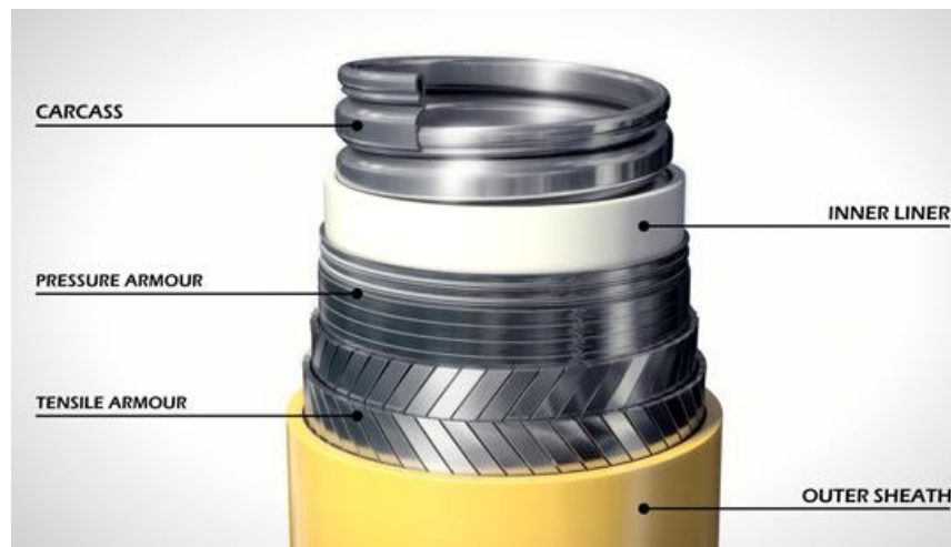
Figure 1 – Typical rough bore flexible pipe build up
