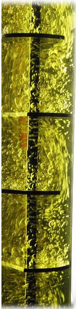
Extraction column for Nuclear-fuel recycling/reprocessing
