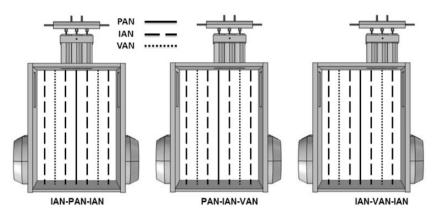
Figure 2. Scheme of the injection system placed on the main cavity roof according to three test configurations.
