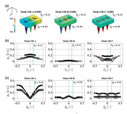
**Figure 5.** Gas dome mode-shapes obtained with COMSOL Multiphysics<sup>®</sup>: (a) real part of the complex pressure amplitude distribution for GD0 ( $d_{or} = 1.125$ ); (b) envelope profiles of pressure amplitudes at  $\tilde{y}_g = 0.16$  w.r.t.  $\tilde{x}_g = x/W_{GD8}$ ; (c) envelope profiles of pressure amplitudes at  $\tilde{x}_g = 0.11$  w.r.t.  $\tilde{y}_g = y/L_{GD}$  ( $\bullet = GD0$ ;  $\bigcirc = GD4$ ;  $\triangleleft = GD8$ ;  $d_{or} = 1.125$ ).
