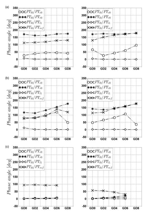
**Figure 11.** Experimental phase-shifts between the  $PT_{10}$  signal and  $PT_{c0}$ ,  $PT_{r0}$ ,  $PT_{11}$ , and  $PT_{ref}$  signals as functions of the dome size, for  $d_{or} = 0.75$  (left side) and  $d_{or} = 1.125$  (right side) at: (a) IAN-VAN-IAN, (b) PAN-IAN-VAN, and (c) IAN-PAN-IAN.
