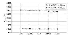
**Figure 8.** Liquid dome eigenfrequencies as a function of dome size  $(L_i = 0.548, d_i = 0.67)$ .
