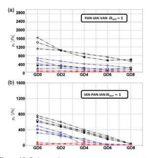
**Figure 10.** Peak-to-peak acoustic pressure measurements in the gas dome as a function of the dome size for the three connection diameters at: (a) PAN-IAN-VAN,  $\tilde{m}_{air} = 1$  and (b) IAN-PAN-IAN,  $\tilde{m}_{air} = 1$  ( $\bigcirc = PT_{10}$ ;  $* = PT_{c0}$ ;  $\diamondsuit PT_{r0}$ ;  $\lhd PT_{11}$ ; red  $d_{or} = 0.375$ ; blue  $d_{or} = 0.75$ ; black  $d_{or} = 1.125$ ).
