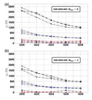
**Figure 9.** Peak-to-peak acoustic pressure measurements in the gas dome as a function of the dome size for the three connection diameters at: (a) IAN-VAN-IAN,  $\tilde{m}_{air} = 0$  and (b) IAN-VAN-IAN,  $\tilde{m}_{air} = 1$  ( $\bigcirc = PT_{10}$ ;  $* = PT_{c0}$ ;  $\diamond = PT_r0$ ;  $\lhd = PT_11$ ; red  $d_{or} = 0.375$ ; blue  $d_{or} = 0.75$ ; black  $d_{or} = 1.125$ ).
