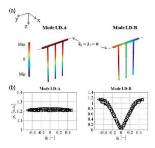
**Figure 7.** Liquid dome mode-shapes obtained with COMSOL Multiphysics<sup>®</sup>: (a) real part of the complex pressure amplitude distribution (*LD*1); (b) envelope profiles of pressure amplitudes w.r.t.  $\tilde{y}_l = y/L_{LD}$  (• = *LD*0;  $\bigcirc$  = *LD*1;  $\triangleleft$  = *LD*2;  $L_j$  = 0.548;  $d_i = 0.67$ ).
