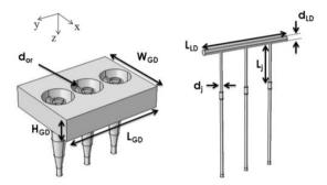
**Figure 3.** Gas dome, *GD*, (left side) and liquid dome, *LD*, (right side) internal domains considered in the numerical simulations.
