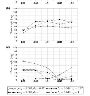
**Figure 14.** Experimental phase-shift between the  $PT_1$  and  $PT_r$ signals as a function of the dome size and  $L_i$  at: (a) IAN-VAN-IAN, (b) PAN-IAN-VAN, and (c) IAN-PAN-IAN.
