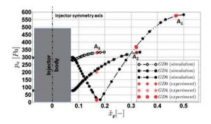
**Figure 12.** Acoustic pressure amplitude with acoustic coupling in the cavity along the gas dome width. Numerical results are compared to experimental measurements (each curve is scaled by the maximum value  $A_i$ , with  $i \in (1,3)$ ).
