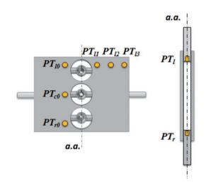
**Figure 4.** Schematic representation of pressure transducer locations in the gas dome (left side) and in the liquid dome (right side). Pressure transducers are represented in yellow.
