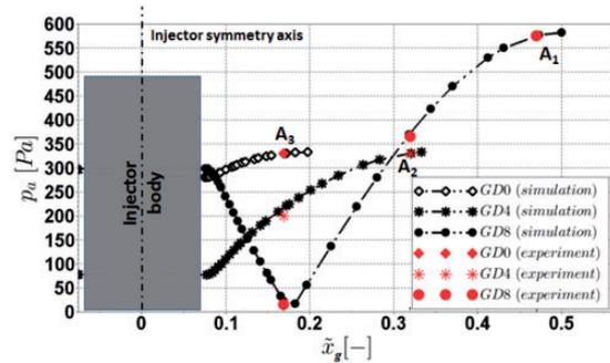
**Figure 12.** Acoustic pressure amplitude with acoustic coupling in the cavity along the gas dome width. Numerical results are compared to experimental measurements (each curve is scaled by the maximum value  $A_i$ , with  $i \in (1,3)$ ).
