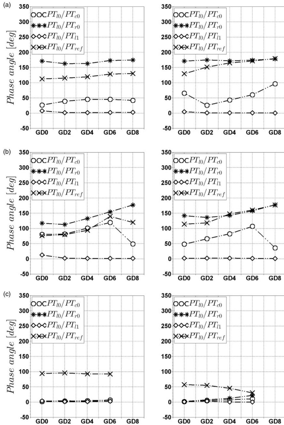
**Figure 11.** Experimental phase-shifts between the  $PT_{10}$  signal and  $PT_{c0}$ ,  $PT_{r0}$ ,  $PT_{l1}$ , and  $PT_{ref}$  signals as functions of the dome size, for  $d_{or} = 0.75$  (left side) and  $d_{or} = 1.125$  (right side) at: (a) IAN-VAN-IAN, (b) PAN-IAN-VAN, and (c) IAN-PAN-IAN.
