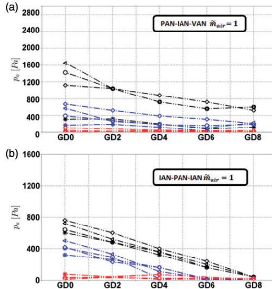
**Figure 10.** Peak-to-peak acoustic pressure measurements in the gas dome as a function of the dome size for the three connection diameters at: (a) PAN-IAN-VAN,  $\tilde{m}_{air} = 1$  and (b) IAN-PAN-IAN,  $\tilde{m}_{air} = 1$  ( $\circ = PT_{I0}$ ;  $* = PT_{C0}$ ;  $\diamond = PT_{I0}$ ;  $\triangle = PT_{I1}$ ; red  $d_{or} = 0.375$ ; blue  $d_{or} = 0.75$ ; black  $d_{or} = 1.125$ ).
