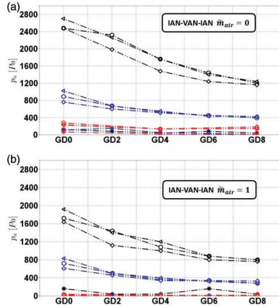
**Figure 9.** Peak-to-peak acoustic pressure measurements in the gas dome as a function of the dome size for the three connection diameters at: (a) IAN-VAN-IAN,  $\tilde{m}_{air} = 0$  and (b) IAN-VAN-IAN,  $\tilde{m}_{air} = 1$  ( $\circ = PT_{I0}$ ;  $* = PT_{C0}$ ;  $\diamond = PT_{I0}$ ;  $\triangle = PT_{I1}$ ; red  $d_{or} = 0.375$ ; blue  $d_{or} = 0.75$ ; black  $d_{or} = 1.125$ ).
