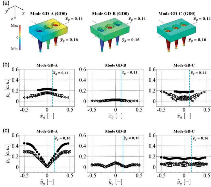
**Figure 5.** Gas dome mode-shapes obtained with COMSOL Multiphysics®: (a) real part of the complex pressure amplitude distribution for GD0 ( $d_{or} = 1.125$ ); (b) envelope profiles of pressure amplitudes at  $\tilde{y}_g = 0.16$  w.r.t.  $\tilde{x}_g = x/W_{GD8}$ ; (c) envelope profiles of pressure amplitudes at  $\tilde{x}_g = 0.11$  w.r.t.  $\tilde{y}_g = y/L_{GD}$  ( $\bullet = GD0$ ;  $\circ = GD4$ ;  $\triangleleft = GD8$ ;  $d_{or} = 1.125$ ).
