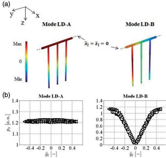
**Figure 7.** Liquid dome mode-shapes obtained with COMSOL Multiphysics®: (a) real part of the complex pressure amplitude distribution (LD1); (b) envelope profiles of pressure amplitudes w.r.t.  $\tilde{y}_l = y/L_{LD}$  ( $\bullet = LD0$ ;  $\circ = LD1$ ;  $\triangle = LD2$ ;  $L_j = 0.548$ ;  $d_j = 0.67$ ).
