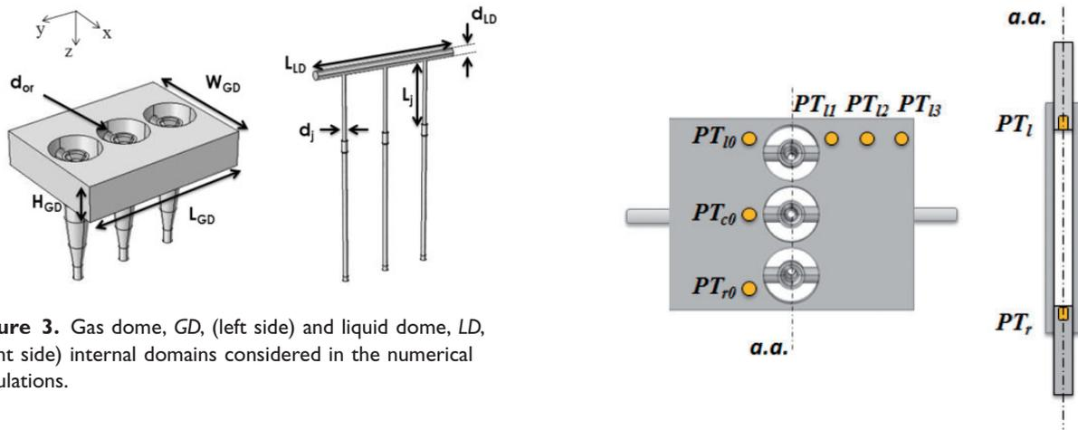
**Figure 3.** Gas dome, GD, (left side) and liquid dome, LD, (right side) internal domains considered in the numerical simulations.
