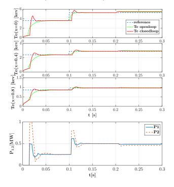
Fig. 5.  $T_e$  tracking and time-evolution of  $P_{1,2}$  when changing the set point and introducing a disturbance at t = 0.2 s in the presence of an input time-delay of 5 ms.
