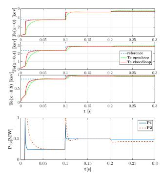
Fig. 3.  $T_e$  tracking and time-evolution of  $P_{1,2}$  when changing the set point and introducing a disturbance at t = 0.2 s.
