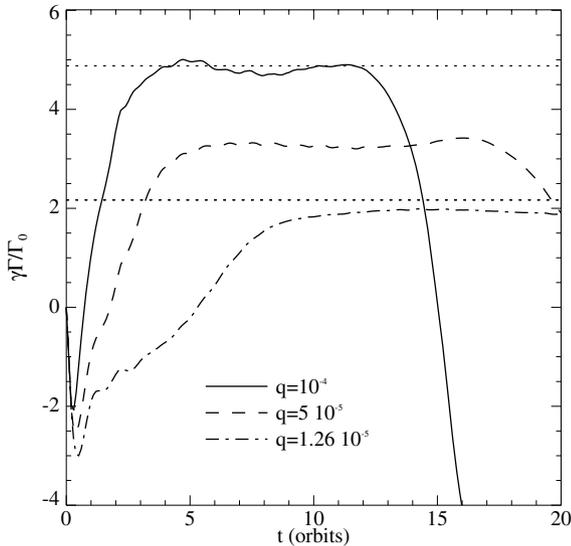
**Figure 17.** Total torque on planets of different masses (using  $b/h = 0.4$ ), embedded in an adiabatic  $\gamma = 5/3$  disc with  $h = 0.05$ ,  $\alpha = 0$  and  $\beta = 1$ . The dotted lines denote equation (47) for  $C = 1.3$  (top) and  $C = 1.1$  (bottom). Results were obtained with `RODEO`.
