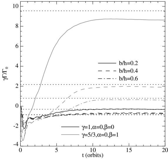
**Figure 14.** Total torque on a  $q = 1.26 \times 10^{-5}$  planet embedded in an  $h = 0.05$  disc with  $\alpha = 0$ , for different values of  $b/h$ , for  $\gamma = 1$  and  $\beta = 0$  (black curves) and for  $\gamma = 5/3$  and  $\beta = 1$  (grey curves). Dotted lines indicate the result of equation (47), for appropriate values of  $C$  and  $d$ . Results were obtained with `RODEO`.
