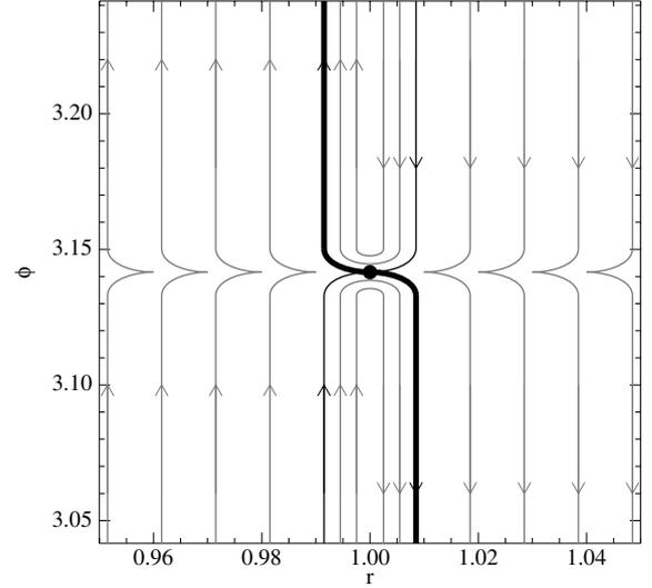
**Figure 4.** Schematic overview of streamlines near the horseshoe region, with the planet indicated by the black dot. The separatrix is coloured black, and the thick curve indicates the location of the entropy discontinuity. The top and bottom of the figure can be thought of as  $\Gamma_2$  and  $\Gamma_1$ , respectively. This picture applies before any material that has made the turn comes back on the other side of the planet.
