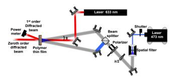
Figure 2: Mach-Zehnder interferometer setup with 1st order diffracted beam measurement
