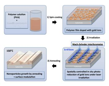
Figure 1: Main steps of the fabrication technique
