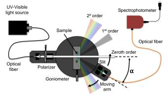
Figure 4: Experiment (2), homemade spectro-goniometer for measuring angular resolved
