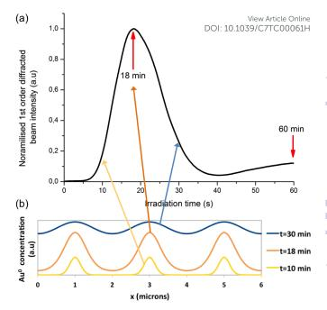
Figure 5: (a) Profile of the first order-diffracted intensity over time during laser irradiation. The maximum of diffraction is reached after 18 min of irradiation. (b) Schematics of the corresponding gold atoms concentration after 10, 18 and 30 min of irradiation.
