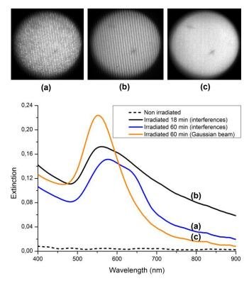
Figure 8: Bright-field images and corresponding extinction spectra of the samples after annealing in the different areas: non irradiated (dashed curve), (a) and (b) irradiated respectively 18 min and 60 min with an interference pattern and (c) irradiated 60 min with a Gaussian beam
