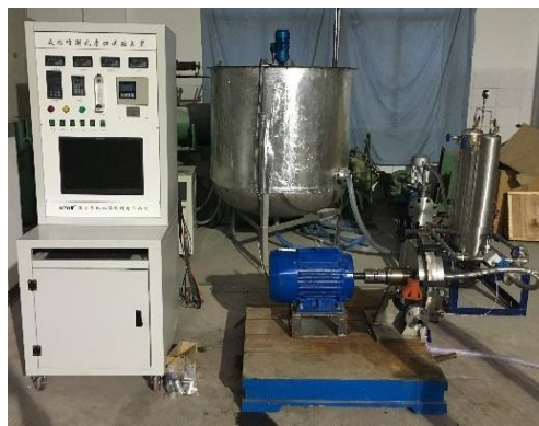
Figure 1. Rotary spray erosion testbed
