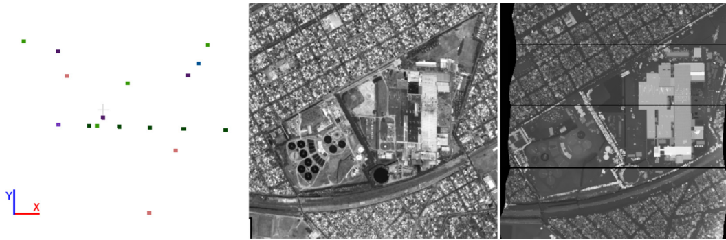
Fig. 6. The MVS benchmark dataset. Left: trajectories of the selected acquisitions; middle: the selected area; right: a LiDAR raster over the selected area.
