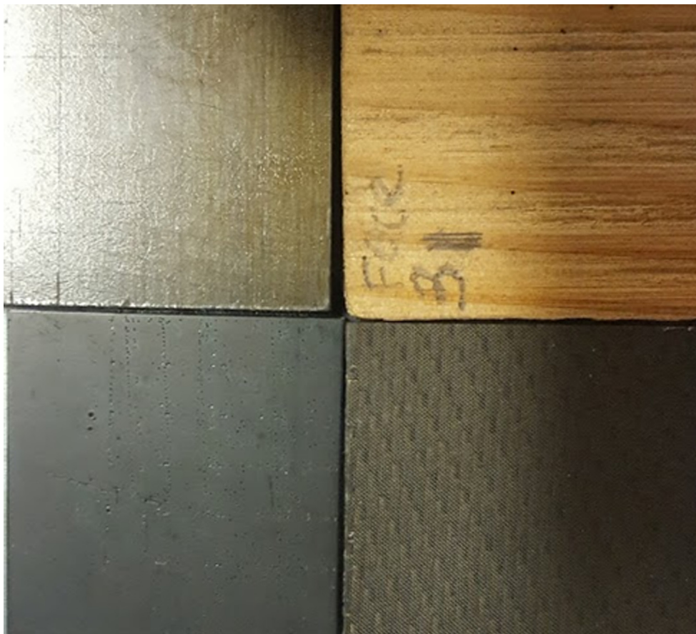
FIG. 2. Heterogeneous sample manually assembled: (a) isotropic carbon/epoxy composite material with fibre tissue, (b) homogeneous and isotropic Plexiglas, (c) pin wood heterogeneous sample with fibres oriented along the x direction, and (d) anisotropic carbon/epoxy composite material with fibres oriented along the y direction.
