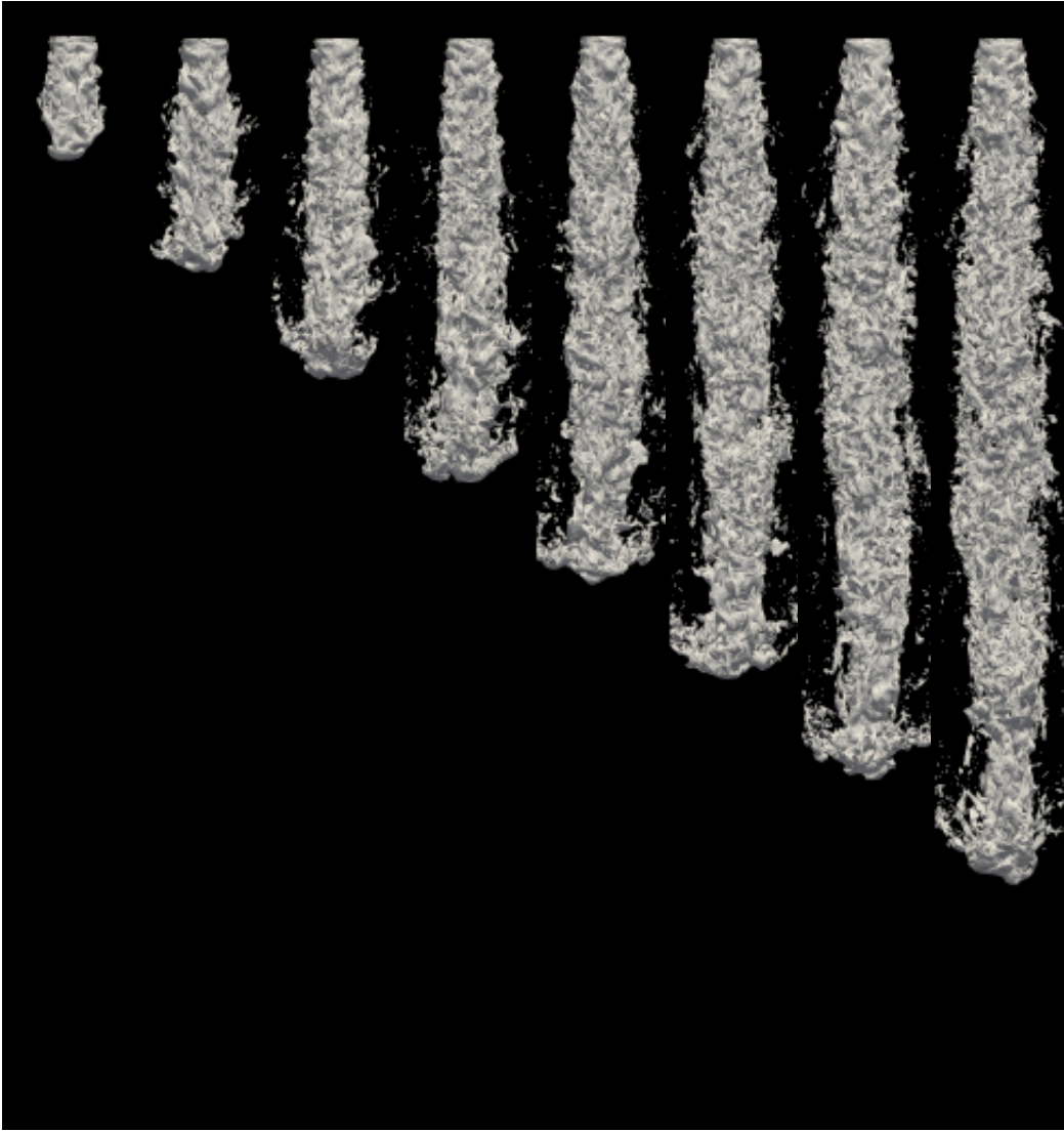
Figure 21: Time evolution of turbulent atomization of liquid diesel jet. \Delta t^* = 2.5 between each snapshot.
